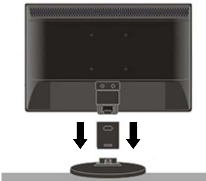
Figure 3-1 Inserting the Monitor into the Pedestal Base
