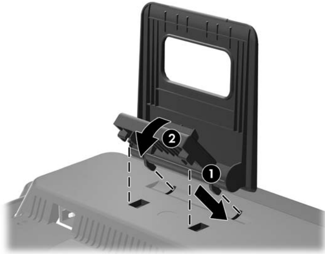
Figure 3-2 Installing the Monitor Stand
