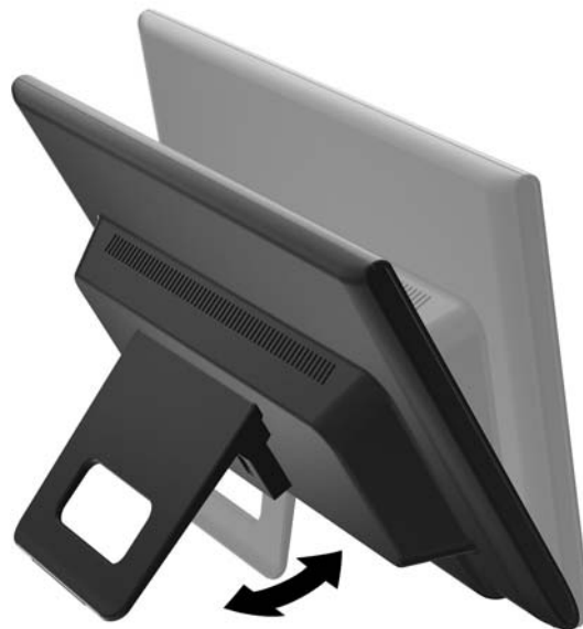
Figure 3-5 Tilting the Monitor
