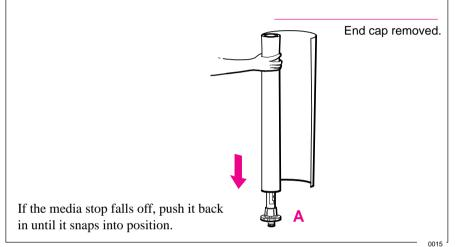
Push the end cap back in, making sure that the tabs are flush against the ends of the roll. Push it far enough to be firm, but do not use excessive force as this may break the tabs.
