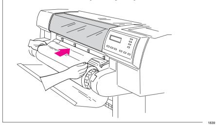
Press the ↓ key next to the front-panel display to indicate you are loading roll media.
