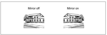
**Do not** change the setting during a plot, as the change becomes effective immediately; if you change the setting in the middle of the current plot, the remaining data is plotted in the mirrored orientation.
