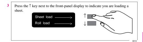
Press the ↑ or ↓ key until the display shows the type of media you are loading (if you are using regular plotter paper, scroll to Opaque bond; if coated paper, scroll to Coated paper), and then press the Enter key.
