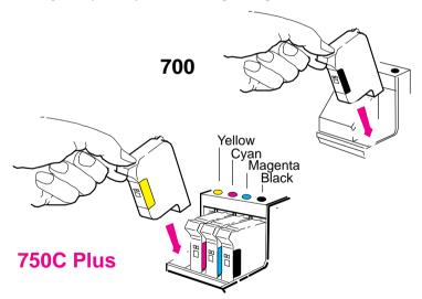
If the front-panel display says Reseat cartridge(s), then remove the cartridge indicated in the display and insert it again. Do so until the message disappears.
