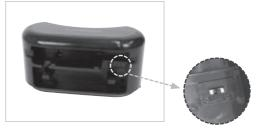
Considering location of the charger and size of the house, set the Sensor Signal Distance Adjustment switch as 5m to 8m to adjust the signal detecting distance of the robot cleaner.
