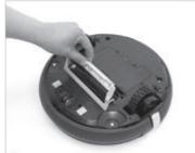
02. Remove the main brush by holding and lifting it.
