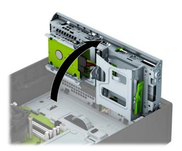
8. Disconnect the power cable (1) and data cable (2) from the back of the hard drive.
