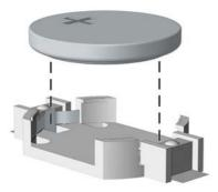
**b.** Slide the replacement battery into position, positive side up. The battery holder automatically secures the battery in the proper position.
