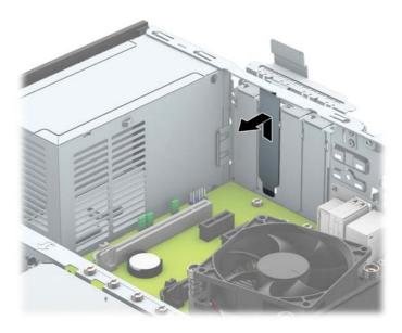
If you are removing a PCI Express x1 card, hold the card at each end, and carefully rock it back and forth until the connectors pull free from the socket. Pull the expansion card straight up from the socket (1) then away from the inside of the chassis to release it from the chassis frame (2). Be sure not to scrape the card against the other components.
