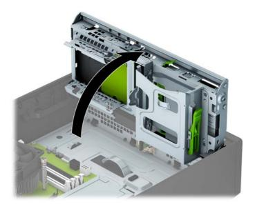
**9.** Align the mounting screws on the drive with the J-slots on the sides of the drive bay. Press the drive up into the drive bay then slide it forward until it locks in place.
