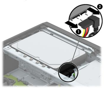
8. Pull the release lever next to the rear of the hard drive outward (1). While pulling the release lever out, slide the drive back until it stops, and then lift the drive up and out of the bay (2).
