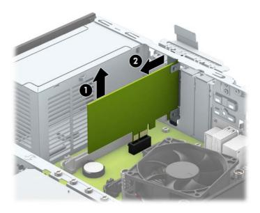
c. If you are removing a PCI Express x16 card, pull the retention arm on the back of the expansion socket away from the card and carefully rock the card back and forth until the connectors pull free from the socket. Pull the expansion card straight up from the socket then away from the inside of the chassis to release it from the chassis frame. Be sure not to scrape the card against the other components.
