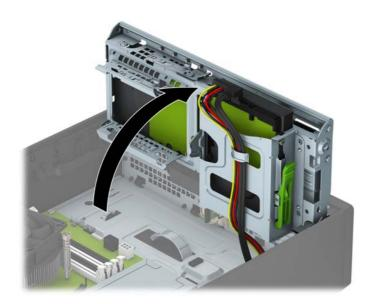
8. Disconnect the power cable (1) and data cable (2) from the rear of the hard drive. Press the latch on the side of the drive cage (3), and then slide the drive out of the drive bay (4).
