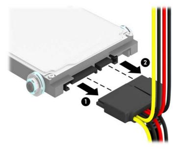
9. Pull outward on the release lever at the rear of the drive (1) then slide the drive back until it stops and pull it down and out of the drive bay (2).
