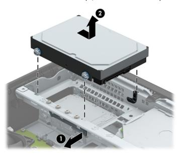
9. To install a hard drive, you must transfer the mounting screws from the old hard drive to the new hard drive.
