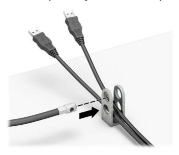
8. Screw the lock to the chassis using the screw provided (1). Insert the plug end of the security cable into the lock (2) and push the button in (3) to engage the lock. Use the key provided to disengage the lock.
