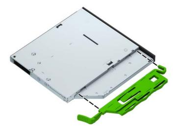
9. Slide the optical drive through the front of the chassis all the way into the bay so that it locks in place (1), and then connect the power cable (2) and data cable (3) to the rear of the drive.
