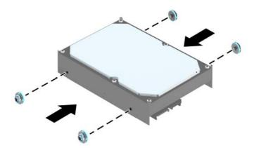
**10.** Align the mounting screws with the slots on the chassis drive cage, press the hard drive down into the bay, and then slide it forward until it stops and locks in place.
