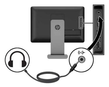
7. Connect the provided audio cable to the audio input connector on the rear of the monitor and the other end to the audio output jack on your input device.
