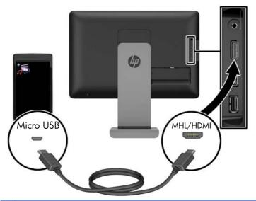
**NOTE:** The MHL/HDMI connector on the side of the monitor is the only connector that is enabled for connecting MHL mobile devices.
