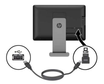
5. Connect a USB device to a USB connector on the side of the monitor.
