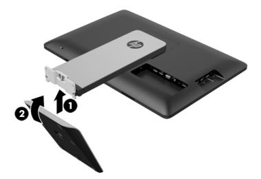
5. Tighten the captive screw on the underside of the base to secure the base to the stand.
