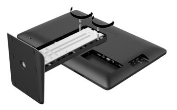
5. Lift the base up after 45 degrees to disengage the stand (1), and then pull the stand off of the monitor (2).
