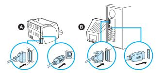
Plug the printer cable into the printer (A). Plug the printer cable into the PC (B).
