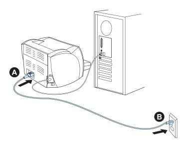
Plug the power cord into the printer (A). Plug the power cord into the power receptacle (B).
