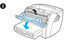
If the printer regularly mispicks (no media feeds through or more than one sheet feeds through), you might need to change or clean the pickup roller. See <u>Accessories and ordering information</u> to order a new pickup roller.
