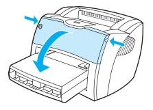
Firmly grasp the left and right sides, and pull the print cartridge door toward you.
