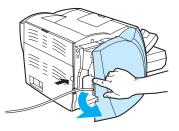
Pull out on the rear of the cover, and rotate it away from the printer.
