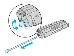
Remove the print cartridge from the plastic bag. To remove the mylar tape, break the tab on the left, and pull the tape completely out.
