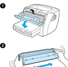
When toner is low, faded or light areas appear on the printed page. You might be able to temporarily improve print quality by redistributing the toner, which means that you might be able to finish the current print job before replacing the print cartridge.
