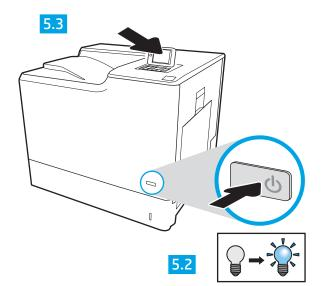
5.1 Connect the power cable between the printer and a grounded AC outlet. 5.2 Turn on the printer. 5.3 On the Initial Setup screen, set the language, the location, the date/time format, and other features.
