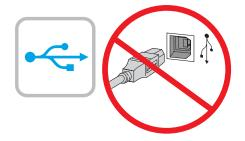
If you are connecting to a network, connect the network cable now. CAUTION: Do not connect the USB cable now. **NOTE**: The cables are not included with the printer.
