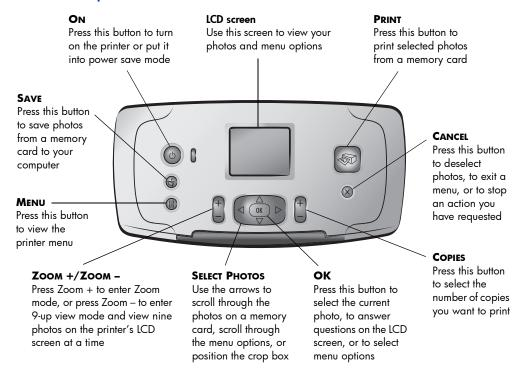
**Note:** The **SAVE** button works only when your printer is connected to a computer. For more information, see the HP Photosmart Printer Help. For information about viewing the Printer Help, see **view the hp photosmart printer help** on page 2.
