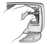
3 Remove the print cartridge from the printer.
