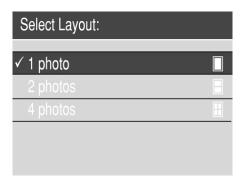
3 Press the SELECT PHOTOS ■ button until the photo layout you want—one, two, or four photos per page—is highlighted on the printer's LCD screen. Press the OK button.
