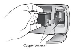
**6** Push the print cartridge into the print cartridge cradle until you feel it snap into place.
