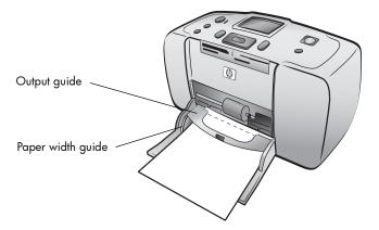
**Tip:** With paper other than HP premium plus photo paper, you may experience paper feeding or ejecting problems. Try loading fewer sheets of paper at a time and make sure the edges of the paper stack are lined up.
