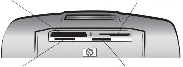
MultiMediaCard<sup>™</sup>/Secure Digital<sup>™</sup> memory card slot You can insert a MultiMediaCard or Secure Digital memory card into this slot
