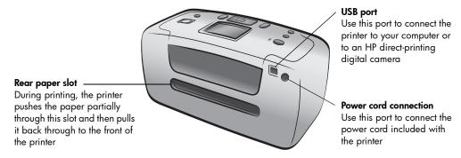
**Note:** Place the printer on a flat, stable surface with the back of the printer at least 10 inches (250 mm) away from any obstruction to allow space for the paper to move during printing. Make sure the power cord and USB cable do not block the rear paper path.
