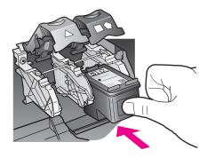
8 Press down on the latch until it stops. Make sure the latch catches below the bottom tabs.
