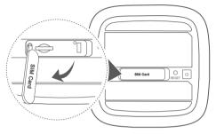
3 Insert the SIM card gently into the SIM card slot in the direction shown in the figure below until it clicks. Then close the SIM card cover.
