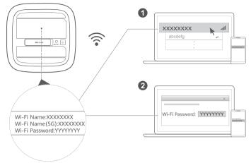
Once the router has connected to a mobile data network, you can connect your computer or mobile phone to the router's Wi-Fi network to access the Internet. Please refer to the label on the bottom of the router for the default Wi-Fi network name (Wi-Fi Name) and password (Wi-Fi Password).
