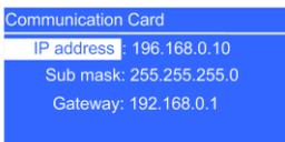
5. On the **Communication Card** screen, set an **IP address**, **Sub mask**, and **Gateway** for the SNMP card.
