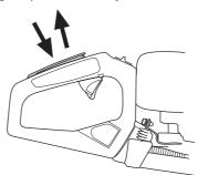
Check that the throttle control and throttle lockout move freely and that the return springs work properly.
