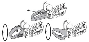
• While working the handle should always be facing upwards irrespective of how the hedge trimmer is directed.
