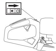
Start the engine and make sure the engine stops when you move the stop switch to the stop setting.
