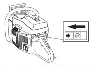
Stop the engine by switching off the ignition. (Move the ignition switch to stop position.)
