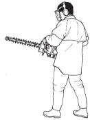
Make sure that your hands and feet do not come near the cutting attachment when the engine is running.
