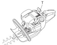
IMPORTANT! If the idle speed cannot be adjusted so that the cutting attachment stops, contact your dealer/service workshop. Do not use the machine until it has been correctly adjusted or repaired.
