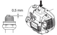
**CAUTION!** Always use the recommended spark plug type! Use of the wrong spark plug can damage the piston/ cylinder. Check that the spark plug is fitted with a suppressor.
