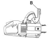
Move the front hand guard forwards and back to make sure it moves freely and that it is securely anchored to the clutch cover.
