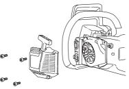
Pull out the cord approx. 30 cm and hook it into the notch in the rim of the pulley. Release the recoil spring by letting the pulley rotate slowly backwards.
