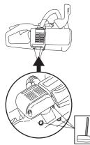
Some mufflers are equipped with a special spark arrestor mesh. If your machine has this type of muffler, you should clean the mesh at least once a week. This is best done with a wire brush. A blocked mesh will cause the engine to overheat and may lead to serious damage.
