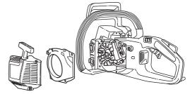
Clean the cooling system with a brush once a week, more often in demanding conditions. A dirty or blocked cooling system results in the machine overheating which causes damage to the piston and cylinder.
