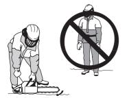
• Always hold the saw with both hands. The right hand should be on the rear handle, and the left hand on the front handle. All people, whether right or left handed, should use this grip. Use a firm grip with thumbs and fingers encircling the chain saw handles.
