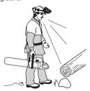
5 Take great care when cutting a tree that is in tension. A tree that is in tension may spring back to its normal position before or after being cut. If you position yourself incorrectly or make the cut in the wrong place the tree may hit you or the machine and cause you to lose control. Both situations can cause serious personal injury.
