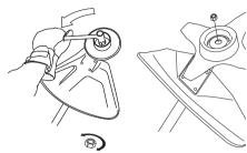
The nylon lining inside the locking nut must not be so worn that you can turn it by hand. The lining should offer a resistance of at least 1.5 Nm. The nut should be replaced after it has been put on approx. 10 times.
