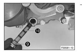
Remove screw plug (9) with oil screen (10) and the O-rings.
