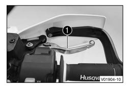
The hand break lever **1** is fitted on the right side of the handlebar.
