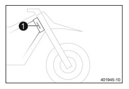
The vehicle identification number ① is stamped on the right side of the steering head.
