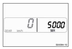
Press the + or - button repeatedly until SER is shown on the combination instrument.
