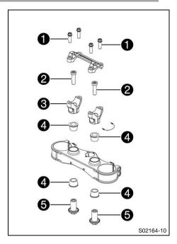
Remove screws **1**. Take off the handlebar clamp. Remove the handlebar and lay it to one side.
