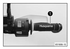
The throttle grip **()** is fitted on the right side of the handlebar.
