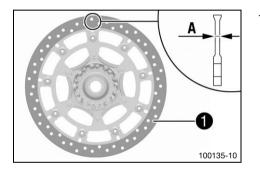
Check the front and rear brake disc thickness at multiple points for the dimension **(A)**.
