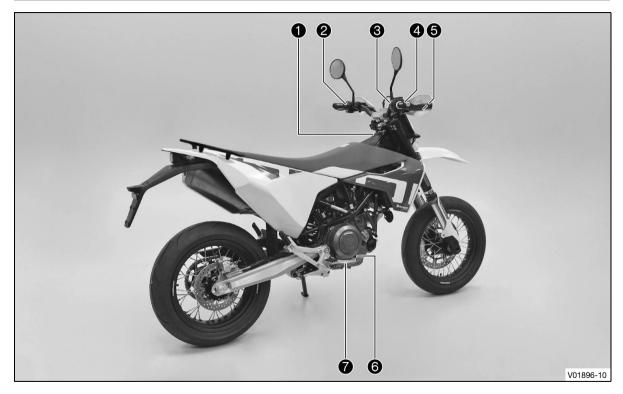
0 Ignition and steering lock (<sup>[2]</sup> p. 34) 0 Horn button (💷 p. 29) 2 Turn signal switch (🕮 p. 30) 2 Light switch (🕮 p. 30) 6 Start button ( p. 32) 6 Emergency OFF switch ( p. 31) 4 Throttle grip (🕮 p. 29) 6 Hand brake lever (🕮 p. 28) 6 Level viewer, engine oil 1 Foot brake lever ( P. 39)
