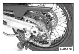
Push the rear wheel forward as far as possible and take the chain off the rear sprocket.
