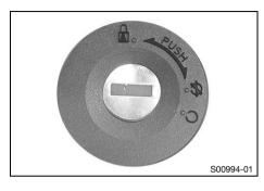
The ignition and steering lock is located in front of the seat.
