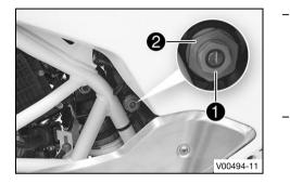
Turn adjusting screw **1** all the way clockwise with a socket wrench.
