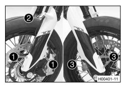
Position the fork protector on the left fork leg. Mount and tighten screws ①.
