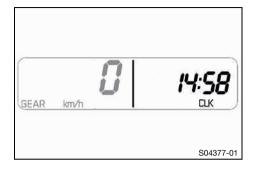
Press the + or - button repeatedly until CLK is shown on the combination instrument.
