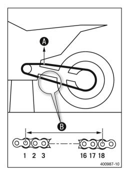
Pull on the top section of the chain with the specified weight A.
