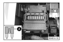
Remove the faulty fuse.
