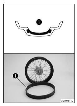
This vehicle uses a tubeless tire system in which a rim seal band **1** is used instead of the conventional tube. The advantages of the tubeless system lie in the absence of danger from a faulty tube. This greatly reduces the risk of a sudden loss in pressure.
