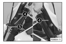
Mount and tighten screws 4.
