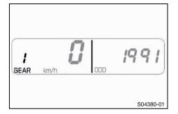
The gear display shows the engaged gear.
