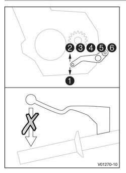
If Easy Shift is activated, you can shift up and down without actuating the clutch.
