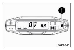
When the fuel level has reached the reserve mark, **TR1 F** appears on the display, and the fuel level warning lamp **1** lights up. This indicator can be closed by pressing the + or - button.
