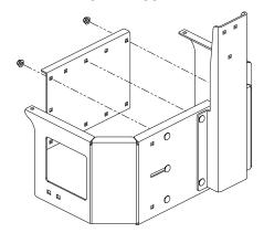
3. Secure collection guard assembly to the mower frame at the side where rear guard was removed. Use two on  $^{3}/_{8}$ -16 x  $^{3}/_{4}$  round head bolts and nuts on each side.
