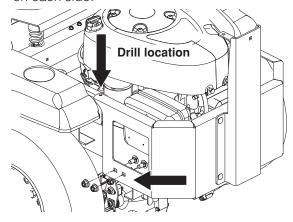
**NOTE**: On some models, it will be necessary to drill a hole in the mower frame to accept the hardware for the collection guard. Use Step 4 for those models. Otherwise skip to Step 5.
