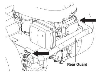
2. Using round head <sup>5</sup>/<sub>16</sub>-18 x <sup>3</sup>/<sub>4</sub> bolts and nuts, assemble the hanger bracket to the rear guard sections and the rear support plate. Use the illustrations for orientation of hardware according to mower size. For the 30" mower, the rear guard sections will fit together. For the 42" mower, the sections will have a gap of approximately 2".
