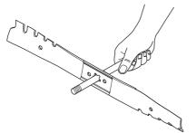
IMPORTANT! The blades should be balanced after sharpening. We do not recommend sharpening blade. Sharpening and balancing the blade should be conducted by an authorized service workshop.
