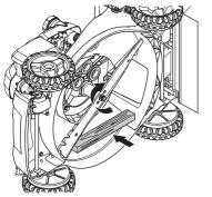
5 The bolt should be tightened with a torque of 35-40 ft. lbs./ 47-54 Nm.
