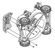
Remove the blade bolt by turning the bolt counterclockwise. Remove blade and attaching hardware: bolt, lock washer and hardened washer.
