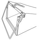
Secure the grass bag to the frame by using the quick-action clips.
