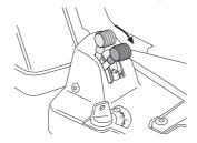
8 Set the required engine speed with the throttle control.
