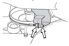
Hold the cable, for example using an adjustable wrench, so that it does not twist.
