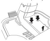
Check the tension of the steering wires by squeezing them together by the arrows as illustrated. It should be possible to push them together so that the distance between them is half as much, without using unnecessary force.
