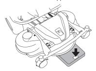
5 Adjust the unit's ground pressure by screwing in or out the adjusting screws located behind the front wheels on both sides. The ground pressure should be between 12 and 15 kg (26.5-33 lb).
