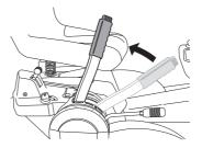
2 Move the throttle control to the MIN. position. Turn the ignition key to the "STOP".
