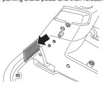
2 Carefully press down one of the pedals until the required speed is obtained. Pedal (1) is used to drive forwards, and pedal (2) to drive backwards.
