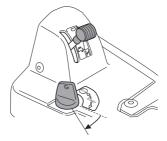
6 When the engine starts release the ignition key immediately back to neutral position.
