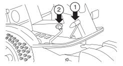
3 Select the required cutting height (1-7) with the cutting height lever.
