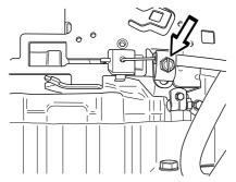
2 Pull the choke wire casing to the far right and tighten the clamping screw.
