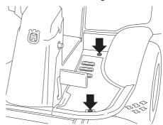
2 Loosen the locking nuts (1).
