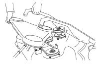
8 Loosen the spring that tensions the V-belt and pry off the belt
