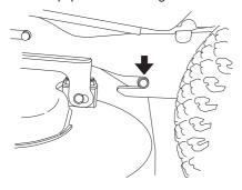
8 Fit the drive belt around the drive wheels of the cutting unit. Make sure the belt is placed on the correct side of the belt tensioner wheel.
