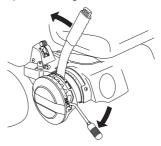
4 Release the clip on the front hood and lift off the fender.
