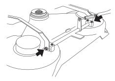
7 Remove the screws on the cutting cover. Lift the unit frame and remove the cutting unit cover.
