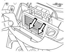
8 Pull the handle outwards. Secure the handle in the air filter cover and close the cover by pressing it inwards.
