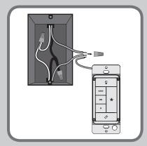
Using orange wire connectors, connect the two black wires (ungrounded) from the outlet box. Also connect the two green or bare wires (grounding) from the outlet box with the grounding wire from the wall control.
