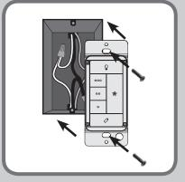
Insert the wall control into the outlet box and secure the two screws using a Phillips head screwdriver.
