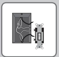
After removing the switch plate cover, remove all wiring from the switch.
