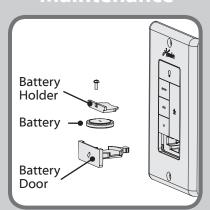
Before operating the wall control, press the battery door to eject it. Using a Phillips head screwdriver, remove the battery holder. Remove the protective film from the battery and install it with the positive (+) side facing downward. Secure the battery by reinstalling the battery holder. Finally, reinstall the battery door into the wall control.
