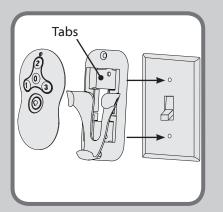
To install the transmitter cradle, remove the two screws holding your switch cover plate. Do not remove the cover plate. Orient the cradle by lining up the two mounting holes with those on the cover plate. Insert and tighten the screws. Do not over tighten. Note: For paddle-style switches, break off the tabs on the cradle by pushing
