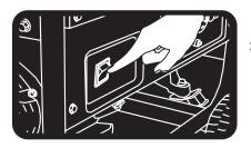
Stop the generator by pressing and holding the engine switch in the "off" position until the generator stops.
