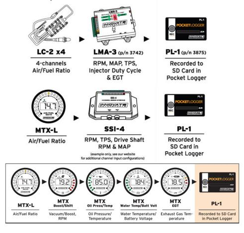
The Innovate Motorsports' MTS (Modular Tuning System) allows you to daisy chain multiple devices (gauges or sensor input boxes) to form one single synchronous log. MTS chains can consist of a single unit connected directly to a laptop, two units, or multiple devices connected together, up to 32 channels.
