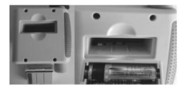
Reinsert the battery housing, ensuring the grooves on the housing and internal section match up. Once the housing is correctly in position, your timer is ready for use.
