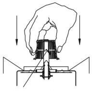
Make this guide coincide perfectly when placing the HydroTurbine in its place.
