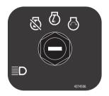
Turn the starter key to the right to start the engine. Release the key to return automatically to the 'on' position for normal operation.
