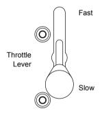
The throttle lever controls the engine speed. Always operate the mower at full throttle during normal operation.
