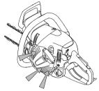
IMPORTANT! In order to maintain operation of the centrifugal cleaning system it must be regularly maintained. Clean the air intake to the starter, the fins on the flywheel, the space around the flywheel, inlet pipe and carburetor compartment.
