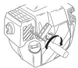
Note that the engine should not be under load when you adjust the high speed jet H. You should therefore remove the cutting attachment, nut, support flange and drive disc before adjusting the high speed jet H.
