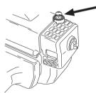
WARNING! When the engine is started with the choke in either the choke or start throttle positions the cutting attachment will start to rotate immediately.
