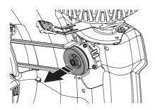
· Pull out the belt and thread it over the adapter.
