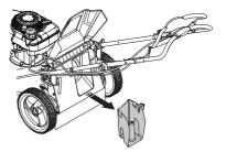
2 Lift the back shield and place the grass catcher frame hooks onto the grass bag brackets.
