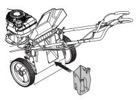
3 Allow the back shield to close and ensure the back shield is firmly shut against the mulch plug.
