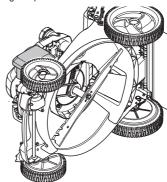
Use a wood block between blade and mower housing to prevent blade from turning when removing blade bolt.
