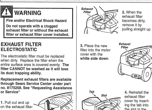
on the exhaust filter cover to remove from the motor cover and lay aside.
