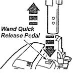
2. Press wand release pedal with foot and pull the wands straight up out of Power-Mate®.
