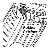
2. Replace the filter, white side out, by sliding it back into place under the ribs in the bag cavity. Tuck filter in so that it fits completely under the rubber retainer.
