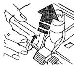
1. Remove light cover by lifting at arrow as shown.
