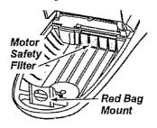
6. Check and replace, if necessary, the motor safety filter. 7. The red bag mount will flip forward after removing bag.
