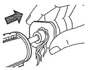
Carefully remove any string or debris located on the agitator, end caps, washers or agitator shaft.
