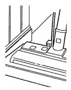
Active brush edge cleaners are on both sides of the Power-Mate<sup>®</sup>. Guide either side of the Power-Mate<sup>®</sup> along baseboards or next to furniture to help remove dirt trapped at carpet edges.
