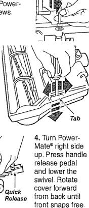
5. Carefully insert and lift screwdriver at each brush support to free brush from base. Brush Support
