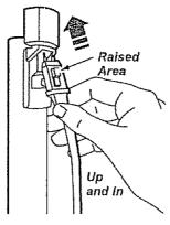
2. Connect Power-Mate<sup>®</sup> plug and cord as shown. DO NOT force. Raised area of plug must be toward hand.
