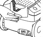
4. Reinstall the exhaust filter cover by inserting the tab into the slot in the motor cover. Press firmly to snap exhaust filter cover into place.
