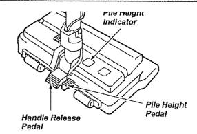
**3.** Lower wand from upright position by pressing on the handle release pedal.
