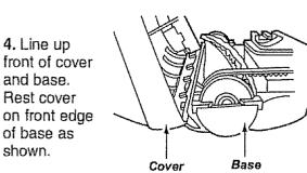
5. Rotate cover back. Press cover firmly until side tabs snap into place. Replace cover screws, light bulb and light cover.
