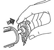
7. Slide brush supports off to check and clean brush support areas. See BRUSH ASSEMBLY for picture of complete brush assembly.
