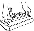
1. Remove light cover by pressing in and lifting both sides as shown.
