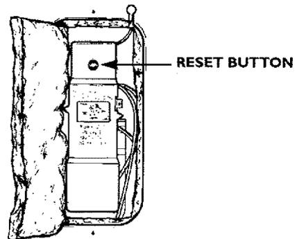
5. Fold the insulation back in place so that it completely covers the thermostat and element.
