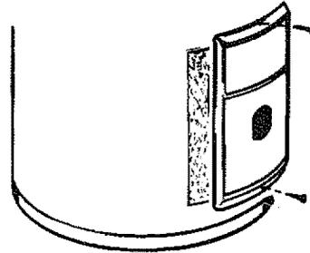
5. Open the flap of insulation to expose the opening.
