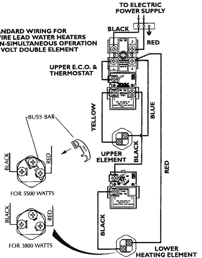
WIRING FOR 3 WIRE LEAD WATER HEATERS
