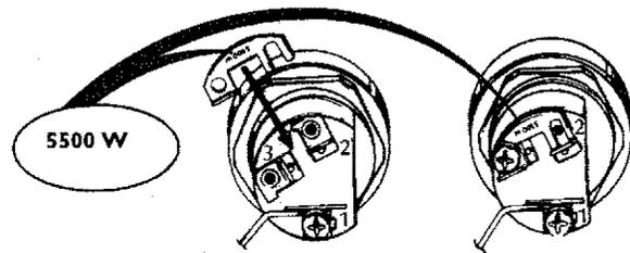
7. The wire removed from terminal 2 has a looped end. It must remain looped and now be placed (as shown) on top of the buss bar, over the opening of terminal 2, and secured using the remaining screw.
