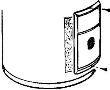
3. Open the flap of insulation to expose the opening.
