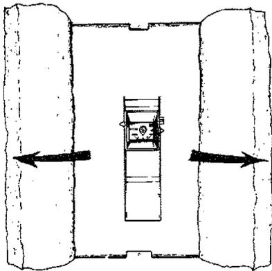
4. **Lower Element:** Lift out the tab as shown to unclip the terminal cover from the thermostat. The terminal cover can now be removed from the thermostat.
