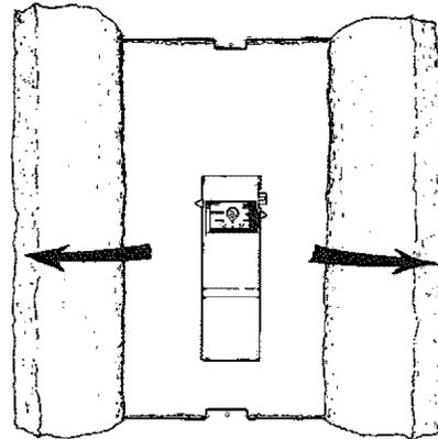
6. Lift out the tab as shown to unclip the terminal cover from the thermostat. The terminal cover can now be removed from the thermostat.
