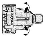
To reassemble, align tabs on the lower housing with the slots on the cover and pivot cover back into position on top of lower housing. Rotate locking tabs inward into locking position.
