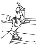
Hold filter under running water to wash. Ring excess water out of filter. Allow filter to dry for at least 24 hours.
