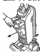
Press dirt container release button and remove dirt container from cleaner.
