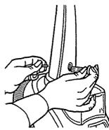
2. Push handle plug onto the front of cleaner. Insert the one (1) screw into the back of the handle and tighten, making sure the handle plug is secure.
