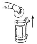
Remove foam filter from dirt container.
