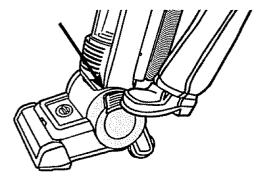
Rotate the handle and adjust it to the desired position for (A) storing the upright, (B) operating the cleaner, and (C) to clean under furniture. **NOTE:** Rotating brush could cause area rug fringe to become tangled within cleaner. Use caution when vacuuming any rugs with fringe.
