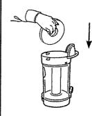
Return filter to dirt container by placing on top of screen inside dirt container.
