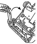
Secure by aligning the three (3) tabs in the base slots. To reattach nozzle guard, rotate/pivot back into position.
