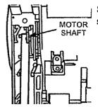
Slide belt onto motor shaft.
