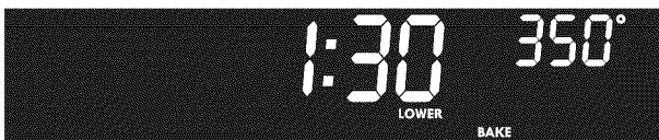
Figure 35: Setting bake for cook time
