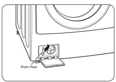
Unclip the drain hose and pull it out. Place the end of the drain hose into a shallow pan or a floor drain. Make sure not to pull the hose out too far, or it may not drain properly.
