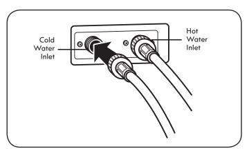
4. Attach the (red) hot water line to the hot water inlet on the back of the washer. Attach the (blue) cold water line to the cold water inlet on the back of the washer. Tighten the fittings securely.
