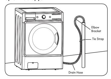
Install the end of the drain hose into the elbow bracket. Do not extend the drain hose more than 4 inches (10 cm) past the end of the elbow bracket. Use a tie strap to secure the drain hose in place.
