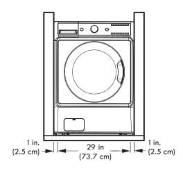
Allow at least  $26^{1/16}$  in. (66.5 cm) in front of the washer to open the door.
