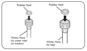
1. Inspect the threaded fitting on each hose and make sure there is a rubber seal in place in both ends.
