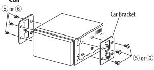
Select the appropriate type of screw for the mounting bracket: flat head (5) or round head (6).
