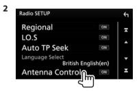
Select this to keep the antenna [NO] extended even when the source is not the tuner.
