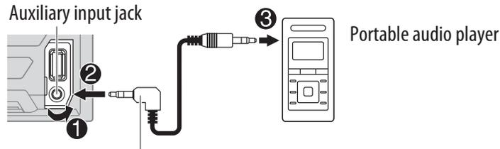
3.5 mm (1/8") stereo mini plug with "L" shaped connector (commercially available)
