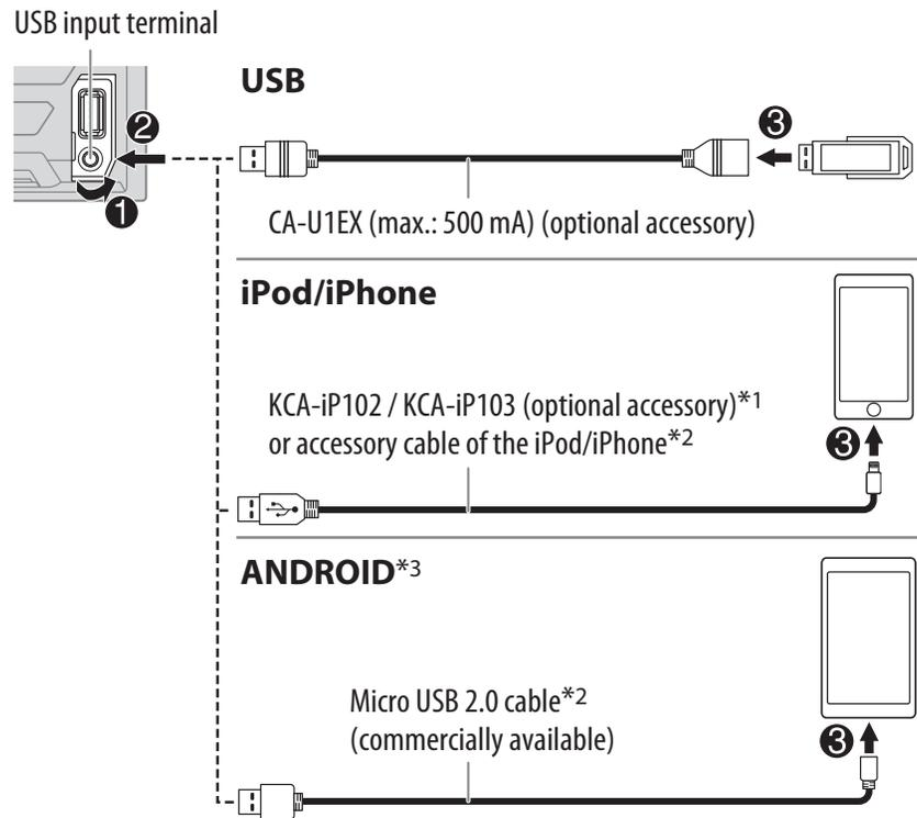
\*1 KCA-iP102 : 30-pin type, KCA-iP103 : Lightning type
