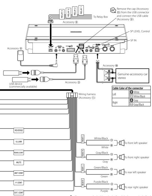
If you connect the ignition wire (red) and the battery wire (yellow) to the car chassis (ground), you may cause a short circuit, that in turn may start a fire. Always connect those wires to the power source running through the fuse box.
