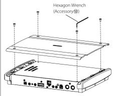
2 Use Tapping screws (Accessory(7)) to fix A/V controller Unit onto an audio board or another. Tapping screw (ø4 × 16 mm)
