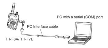
For your information, the following diagram shows how the TH-F6A/TH-F7E communicates to the PC using a serial (COM) port.
