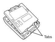
4 To install the battery case onto (or remove it from) the transceiver, follow steps 1 to 3 of "INSTALLING THE Li-ion BATTERY PACK" {above}.
