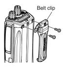
If necessary, attach the belt clip using the two supplied M3 x 8 mm screws.
