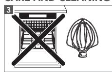
**IMPORTANT:** The Wire Whip is only dishwasher-safe for models 5KSM200, 5KSM185, and 5KSM180. For all other models: Wash it thoroughly in hot sudsy water and rinse completely before drying. Do not store Wire Whip on shaft.
