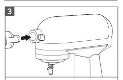
Insert the attachment shaft Housing into the attachment hub.
