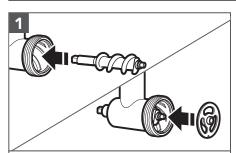
Insert the Grind Screw into the Main Housing. Then insert the Sausage Stuffer Plate over the end of the Grind Screw, matching the notch of the plate with the tab on the bottom of the Main Housing.
