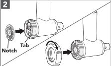
Place the desired Grinding Plate over the Blade, matching the notch of the plate with the tab on the bottom of the Main Housing.
