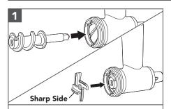
Insert the Grind Screw into the Main Housing securely. Place the Blade over the end of the Grind Screw.
