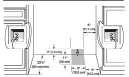
If water shutoff valve is located in base cabinet, access hole through side of cabinet must be within 1/2" (12.7 mm) of rear wall. Right side cabinet is recommended. If water shutoff valve is not in cabinets, water line can come through rear wall or floor in shaded area dimensioned above.
