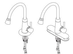
Attach cover plate to bottom of faucet with bottom Note: If the sink is with two holes , the cover plate is not installed. Attach body trim ring to bottom of
