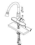
Place silicone sealant beneath the bottom plate and install faucet through center
