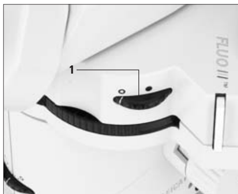
Fig. 7 1 On/off switch for UV shutter
