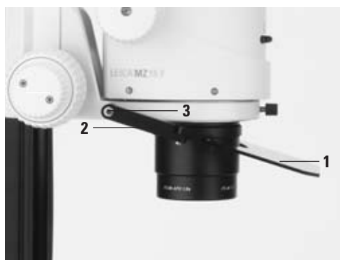
Fig. 5 UV protection screen 1 UV protection screen 2 Arm 3 Hexagon-head screw
