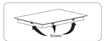
2 Carefully lower the cooktop into the counter- top cutout, making sure not to trap any wires. NOTE: Do not use caulking compound. The cooktop must be removable, should service be required.
